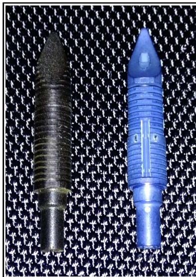
Fig.-2, The new replacement Ebonite feed (left), and the original 743/FA plastic feed (right).
