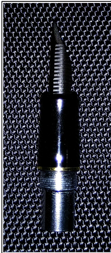
Fig.-4, The assembled feed and seal-washer (without the nib) properly inserted into the section. Note there are thirteen (13) exposed feed fins above the end of the section in this particular example.
