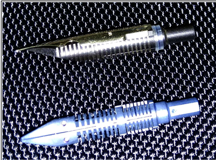
Fig.-3, Top: The original FA nib and rubber seal-washer installed on the new Ebonite feed. Bottom: The original bare plastic feed.
