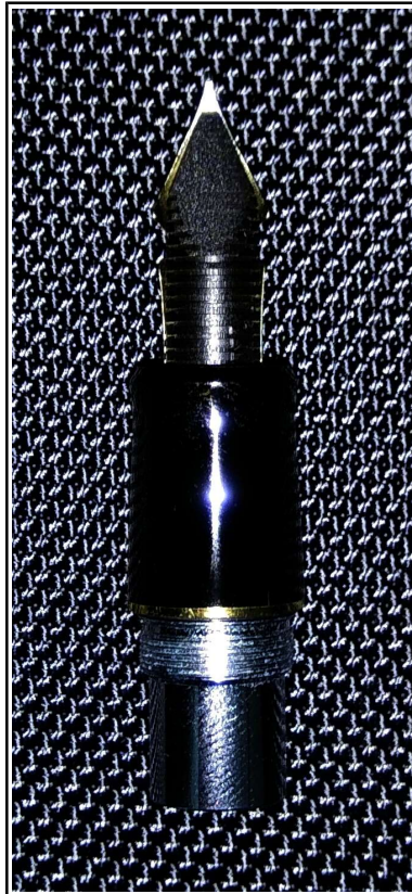
Fig.-5, The fully assembled nib, new Ebonite feed, and seal-washer. Note the thirteen (13) exposed feed fins, the same number as seen in Fig.-4.
